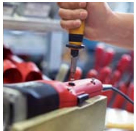
Assembly of the individual components, including the housing, motor and electronic unit.
