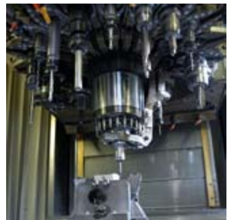
State-of-the-art five-axis machining centre: ultra-precision machining of gear housings.
