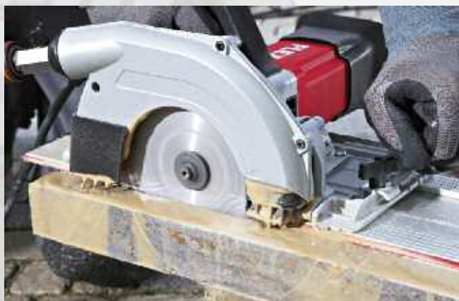
A long service life: the water feed, which effectively cools the diamond cutter, while the rubber end sleeve protects the motor from spray water ingress. A GFCI operator protector circuit breaker, built into the cable ensures safety when wet cutting.
