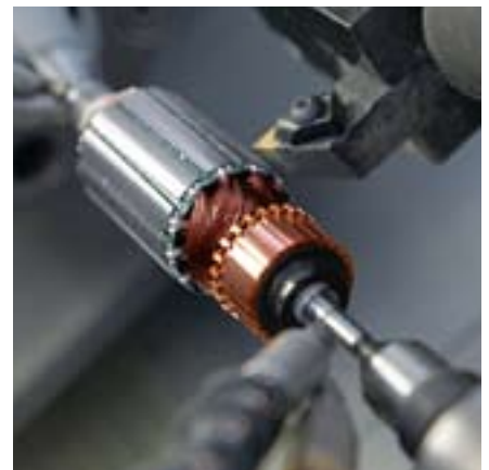
Maximum precision: anchors are fully machined in a single chucking operation.
